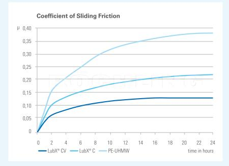
The tests were carried out at the company's materials laboratory on a tribology test apparatus developed in co-operation with scientists. In order to adapt the test procedure to the increased requirements, the conditions were significantly increased for the application-oriented test: The speed was doubled to 0.5 m/s and the surface pressure was doubled to 0.5 MPa.
