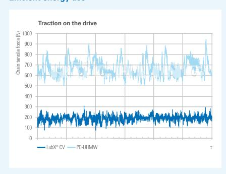
To measure the tensile force on the drive LubX® CV was tested in comparison with a standard PE-UHMW on an application oriented conveyor belt system.
