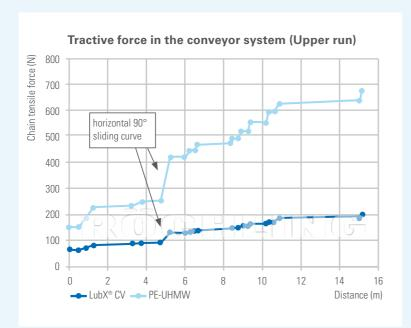
The graph shows the theoretical tractive force development within a complex conveyor belt system utilizing LubX® CV and PE-UHMW chain guides under the assumption of the measured coefficient of sliding friction. The curved areas within the test section can be clearly identified by the increase in tractive force in the graph. The flat tractive force development utilizing LubX® CV on the entire track conserves the conveyor chain and contributes to a high process stability.
