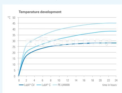
During the test of the coefficient of sliding friction, an infrared sensor (pyrometer) measures the temperature development directly on the friction surface of the sample without contacting it. The measured temperature of LubX® CV in the test does not rise over 28° C, which was up to 17° C below the other material samples. In addition, the LubX® CV sample shows almost **no signs of wear** after 24 hours.
